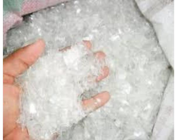
This recycled and cleaned material — the washed PET flakes — is thus ready for further manufacturing use without compromising on quality.
